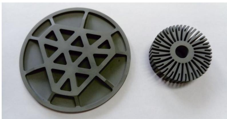
Figure 2 Parts printed by 3DCERAM with  $\text{Si}_3\text{N}_4$  ceramic (after sintering) (© 3DCeram Sinto)
