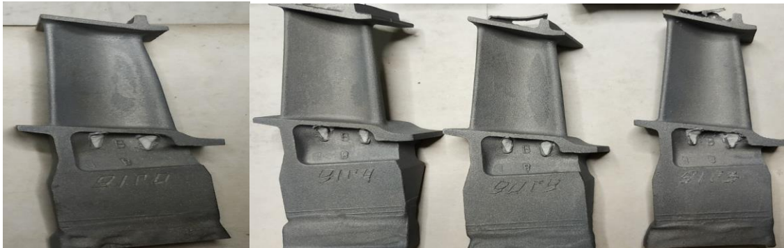
Foundry moulds (Ni-alloy with Silicore cores).
