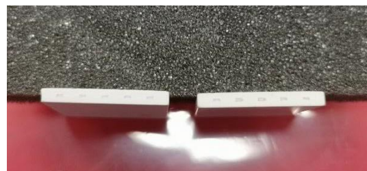
After printing and cutting the part, we can observe the internal cannels made with polymerized resin
