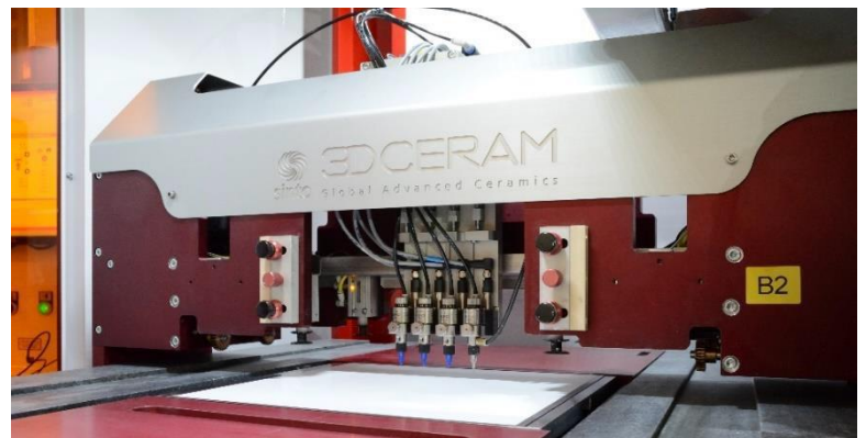
Nozzle system on the C900 for multi-material printing
