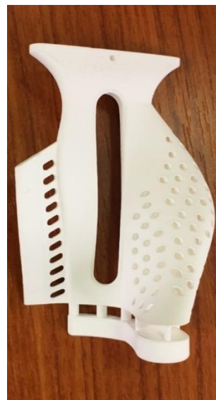
Part after printing and firing
