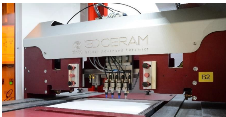
Nozzle system on the C900 for multi-material printing
