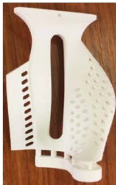
Fig. 6 Core after printing and firing
