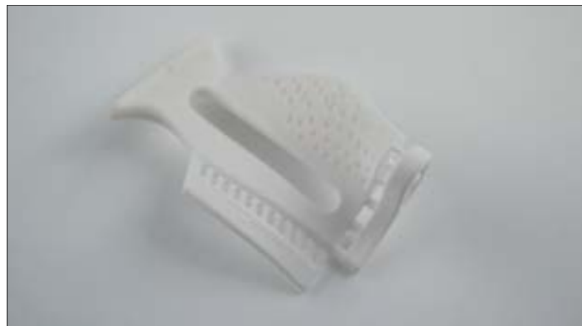
Fig. 1 A new generation of foundry cores produced by 3D Printing
