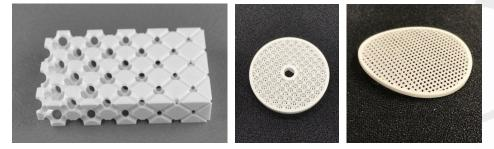
The risk analysis is completed by a proposition of benchmark to mitigate the risk. This simple printed benchmark can evaluate the risk and define the best way to produce the final part.
