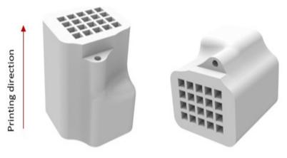
In this case, we did some CAD proposals to make it more robust. The main objective of this step is to reduce the default (scratch, failure...) which can appear during the process. We start by the choice of the **part orientation** which depends to the **part tolerances** and the target unit price. An example is presented hereafter on a simple part. In this case, the vertical part will be more precise than the other orientation, but the printing time (and the cost) will be higher.
