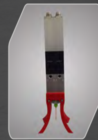
Extrusion (Robocasting for 2 components)
