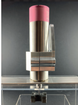
CNC Tool 3-axis CNC tool for green machining of printed parts before firing
