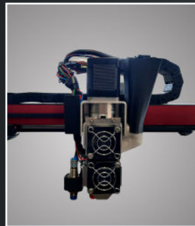
Direct Pellet Extrusion (DPE) Head for working with ceramic and metal pellets
