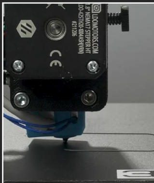
FFF Head for working with ceramic and metal filaments
